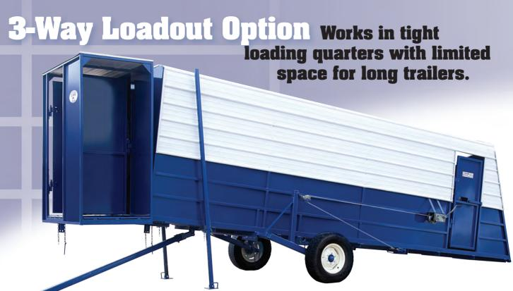
This Option allows amimals to exit to the trailer either to the left, to the center, or to the right. Two hinged door panels swing and lock to make the exit direction change convenient.
